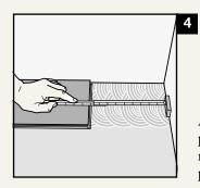
At the end of the first row, put a wedge to the wall and measure the length of the last plank to fit.
