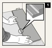
First plank, first row. Start in the left corner with the tongue side facing the wall and the long groove side directly up against the straight edge. Spread enough adhesive to cover one plank width. Use only as much adhesive as can be used during the manufacturer's maximum recommended time for keeping the container open.
