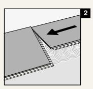
Second plank, first row. Line up the plank gently and tightly to the short end of the previous plank.
